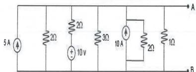
b Find the Norton's equivalent across AB for the given circuit. CO1 L3 5M
